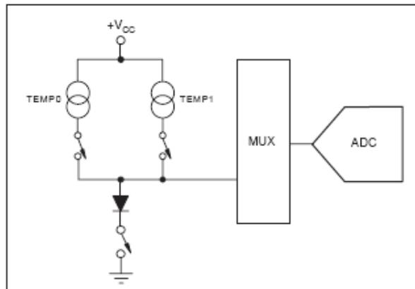
Figure 6. Functional Block Diagram of Temperature Measurement
