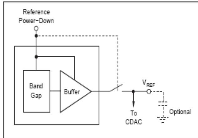
Figure 3. Simplified Diagram of the Internal Reference
