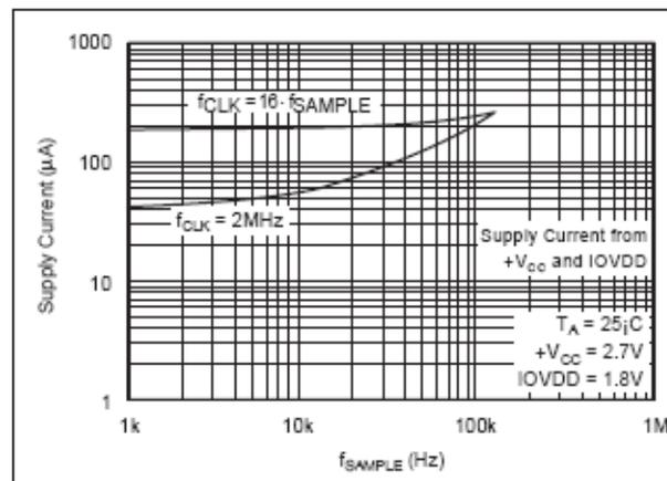
Figure 15. Supply Current versus Directly Scaling the Frequency of DCLK with Sample Rate or Maintaining DCLK at the
